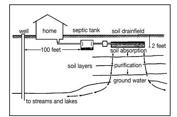
Figure 3 Wastewater Treatment and Disposal In the Soil Courtesy-North Carolina Extension Service
