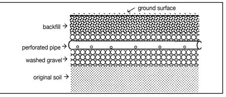
Figure 4 Septic Drainfield Courtesy–Washington State University
