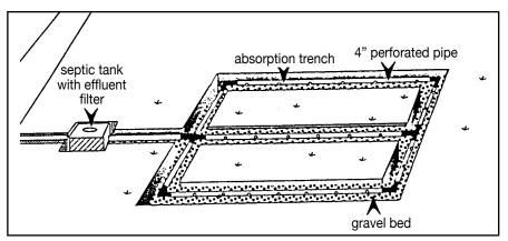
**Figure 1: Septic System with Effluent filter**—The Montana Waste Water Association requires effluent filters and risers of at least 21" diameter to w/in 6" of grade. Risers must have a shut off (float ball) built in so nothing will pass through if the filter cartridge is removed. When a riser is installed, it replaces the concrete lid and a new lid is placed at grade. Courtesy National Small Flows Clearinghouse \*
