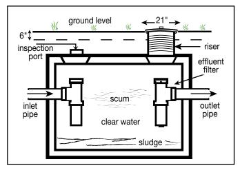
Figure 2: Septic Tank with Effluent Filter
