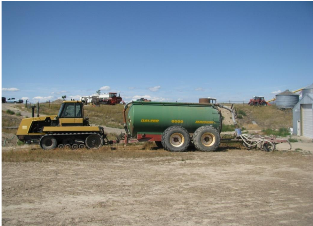
Figure 27. Septage Injection System Designed by a Landowner in the Amsterdam Area. This is the only septage injection system known in the area.
