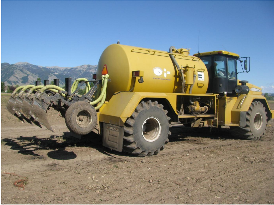
Figure 30. Biosolids Injector Truck used by the City of Bozeman Wastewater Treatment Plant. The Bozeman has the largest, and the most structured program for handling and disposing of biosolids. Specialized trucks inject the biosolids into the soil.
