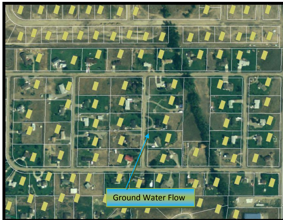
Figure 34. Visualization of Mixing Zones for Individual Septic Systems in a High Density Area. The yellow rectangles are the surface areas of the mixing zones, oriented with ground water flow.
