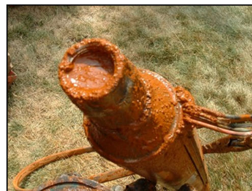
Iron bacteria can cause a nuisance, rust-colored, slimy biofilm.
