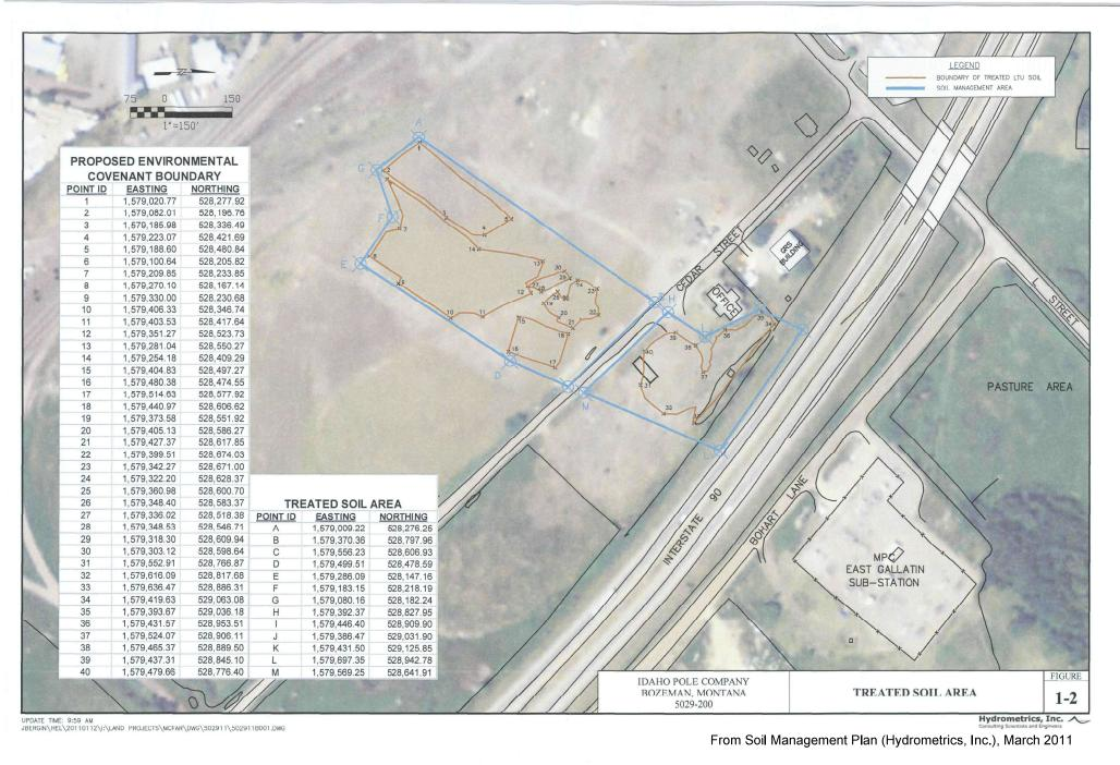
Figure 4. "Treated Soils Areas" Where Treated Soils Were Placed Onsite
