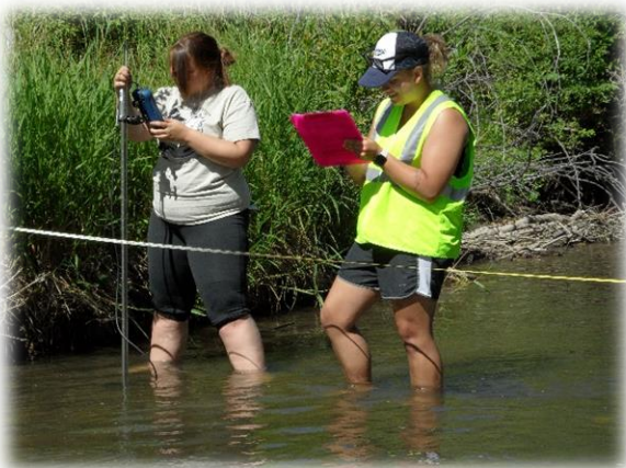
Figure 4. Gallatin Stream Team citizen scientists measuring stream discharge on the East Gallatin River at the Story Mill Community Park site.
