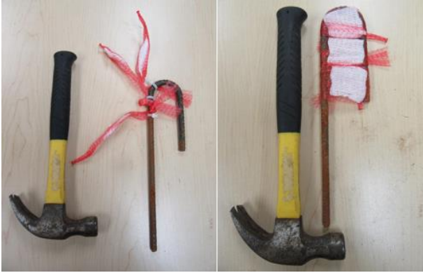
Figure 5. OB pad deployment setup for Sampling Event 1 (left) and as modified for Sampling Event 2 (right).
